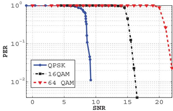
Fig. 13: Packet Error Rate vs SNR for Various Modulation Schemes
