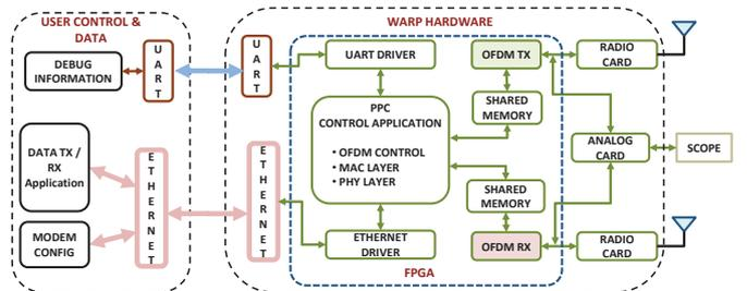
Fig. 6: Detailed Hardware Architecture of Hardware Test Bed
