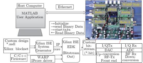
Fig. 8: Design Flow in WARP
