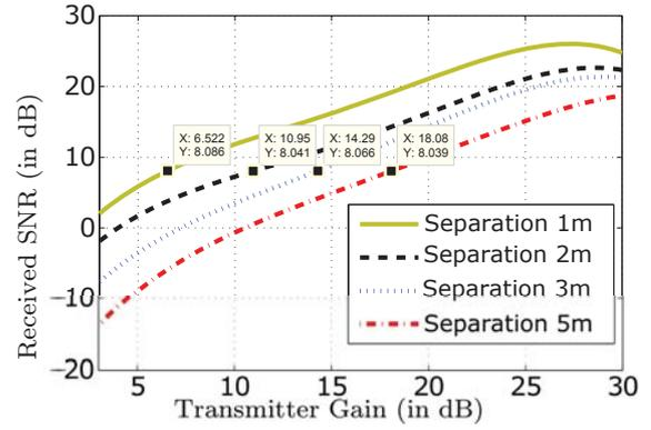
Fig. 10: Received SNR vs Transmitter Gain for Various Distance
