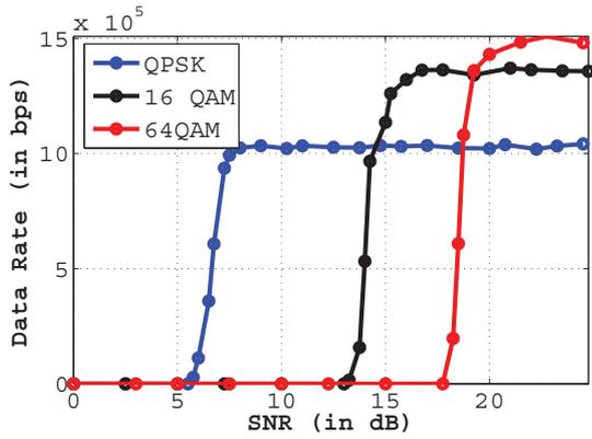
Fig. 12: Data Rate vs SNR Performance for Various Modulation Schemes
