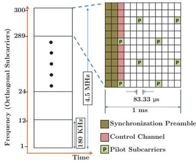
Fig. 4: Frequency Domain Packet Format
