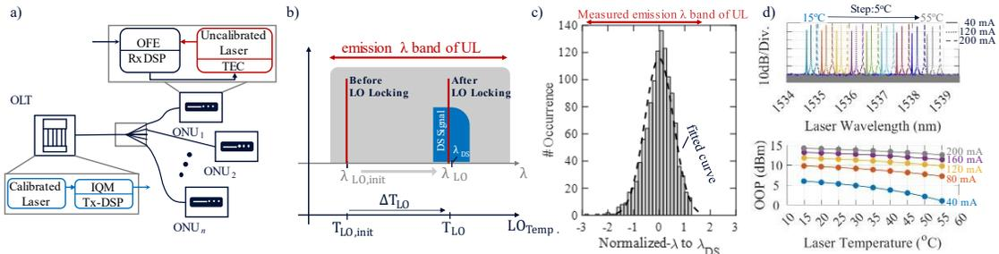
Fig. 1. Potential architecture for VHSP. (a) Coherent PON using an uncalibrated LO laser at the ONU side. OFE: optical front-end. (b) Illustration of the  $\lambda$  ambiguity for the uncalibrated laser (UL). (c) The histogram of the measured emission wavelength of over 1000 DFB lasers. (d) Characteristics of the DFB laser used in the experiment for different operating temperature and bias current.
